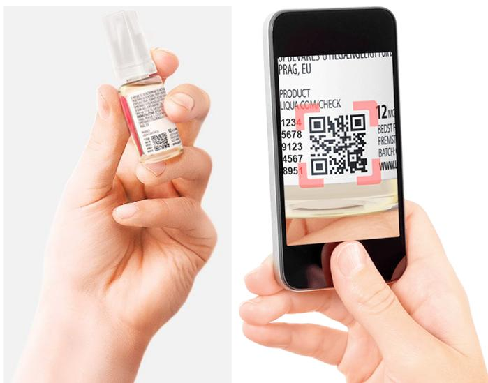
From 2014 Ritchy uses a security and batch tracking system developed in-house. Every single product produced from that time (and at this moment - all products in service) is stored in the database with 2D codes available for consumers. That can be used to validate that the product is genuine (# of checks is limited, so any counterfeit products run out of codes) and to have a connection directly to the consumer.
